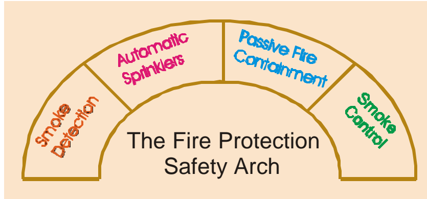
Figure 1 - Effective fire protection requires a systems approach with four primary elements in place, installed in accordance with established standards, and monitored for continuing effectiveness. Sprinklers alone cannot effectively protect life and property.
